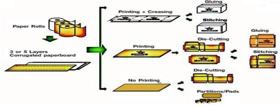
Printing is performed on corrugated box blanks that have been formed, scored and cut by a corrugator. The box blanks are subsequently cut or Die-cut into specific shapes for further forming into finished boxes. Printing Machine require 2 main operator and 6 helper in order to match the speed of the production
